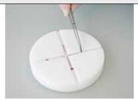
Adjust the second MTS (antibiotic B) such that the MIC value of the second antibiotic (MIC<sub>B</sub>) is positioned at the base intersection and intersects MTS-antibiotic A at its MIC value.
